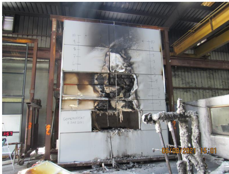
Photo No. 2 Armatherm Z-Girt assembly after test. (Panels were removed to extinguish fire after the test).
