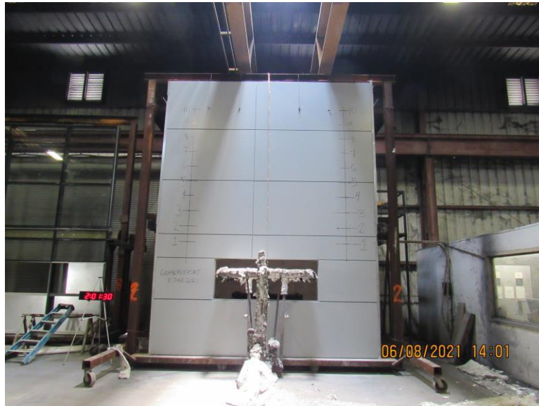
Photo No. 1 Armatherm Z-Girt assembly before test.
